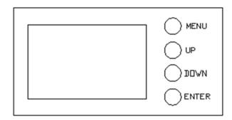
To view or modify the function settings of the lamp, press any key (in the power-on state) to light up the screen, and then press the UP and DOWN keys to enter the corresponding menu of the lamp. There are corresponding sub-menus in the function operation main menu, and each menu represents a specific function of the lamp. For details, see the sixth point "Operation Menu" below.
